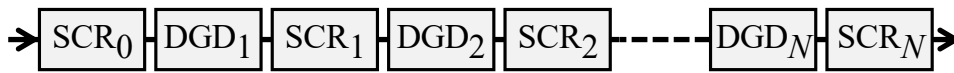
PMD emulator with N DGD sections (indices 1... N ) placed between N+1 retarders/scramblers SCR (indices 0... N )
