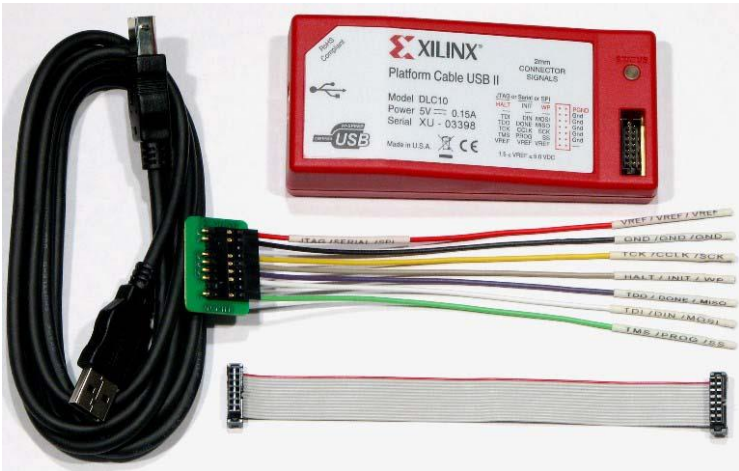
Fig. 1: XILINX Platform Cable USB II
